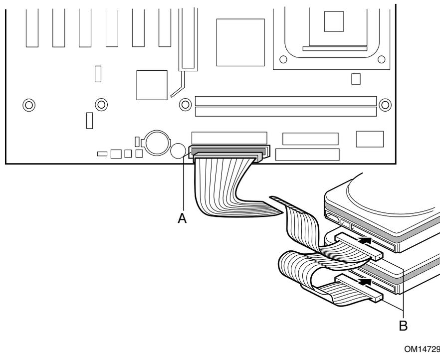
**Figure 9. Connecting the IDE Cable**
